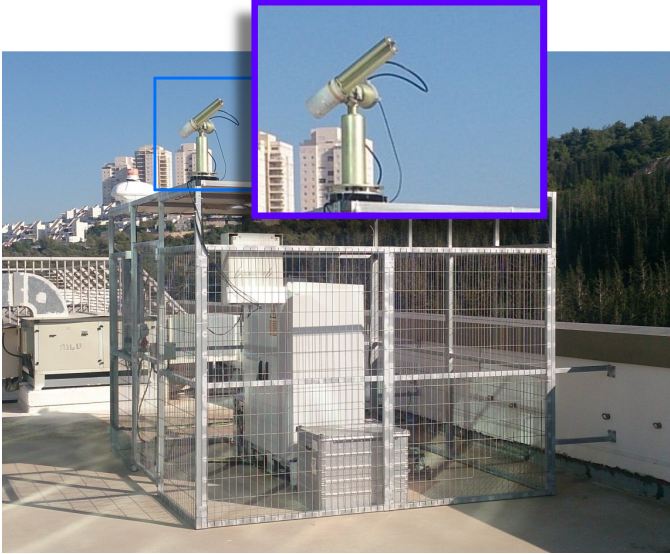
Figure 3: The Raman aerosol lidar used during our experiments. It is the PollyXT system by TROPOS, installed on the roof the Meyer (EE) Building, Technion, Haifa, Israel. The AERONET sunphotometer can be seen on top of the installation cage.
